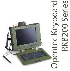
Designed to meet Temp operating Temp storage Dimensions ( $W \times D \times H$ ) Weight 66 key B/L, Elastormer keys (backlight), USB IP54, MIL-STD-810G -30° to +55 °C (-22°F to +132°F) -40° to +70 °C( -40°F to +158°F) 235 × 200 × 15.5 mm (9.25 x 7.87 x 0.61 in) <0.7 kg (1.54 lbs)
